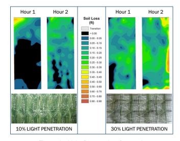
Figure 1 - Light Penetration Comparison
