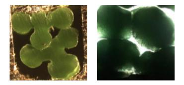
Figure 2 - Trilobal Fiber (Left) vs. Round Fiber (Right)
