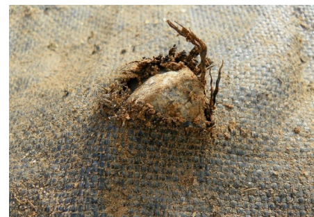
Figure 14 - Woven tearing over rock
