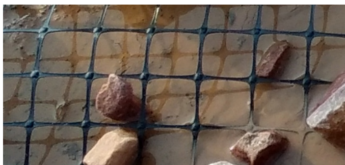
Figure 4 - Geogrid aperture size
