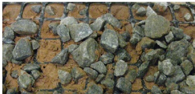
Figure 5 - Geogrid aperture size
