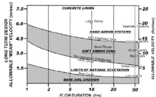
Figure 2 - Allowable velocities and flow duration for various erosion and bank protection measures
