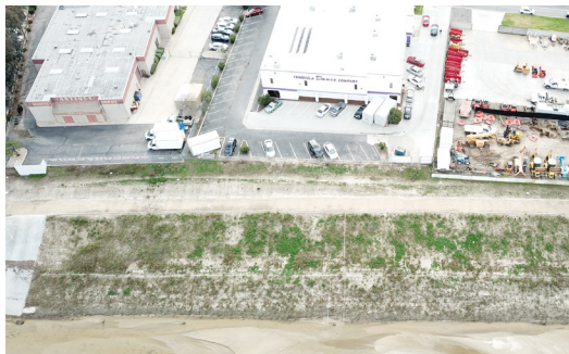
PROBLEM Erosion and scour of Murrieta Creek banks due to flooding events
