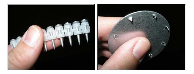
6. If during installation of the concrete interlayer geotextile, the nail does not fully penetrate the existing pavement, drive another nail and washer next it.
