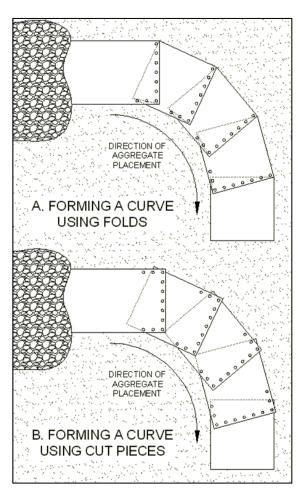
(Note: o – indicates location of pins, sandbags, piles of fill or rock, or other means of temporarily anchoring geotextile.)
